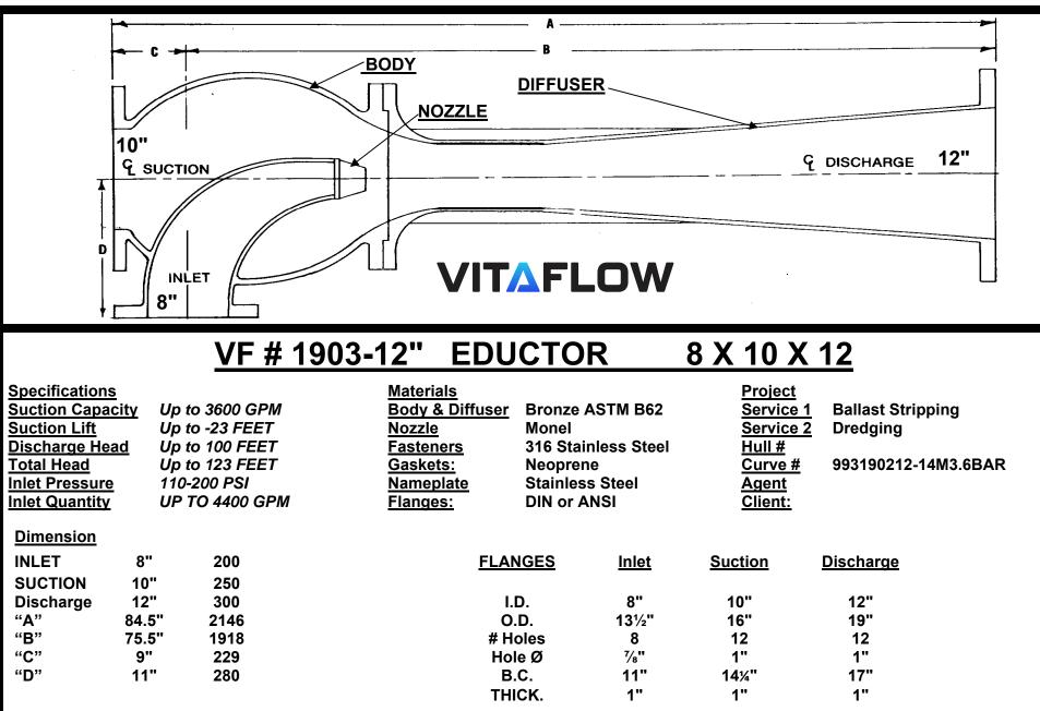
1. Eductor is supplied to meet the requirements of each application. Customer should follow the VM installation, technical and maintenance manual.
