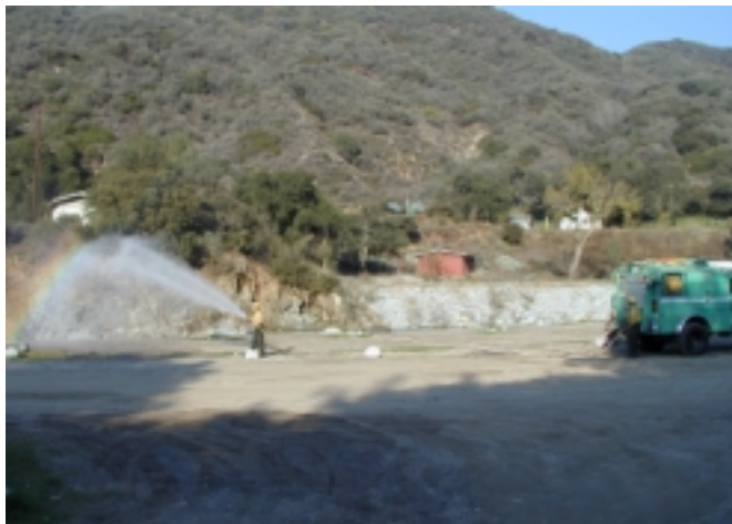
Figure 4—Ejector drafting operation to support fire suppression and maintain a full tank.
