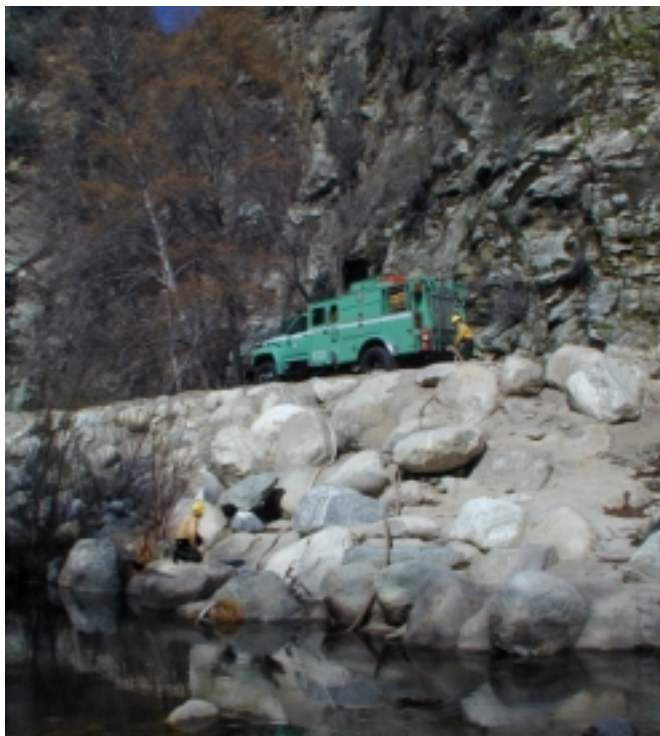
Figure 5—Ejector drafting operation at a lift greater than 22 ft.
