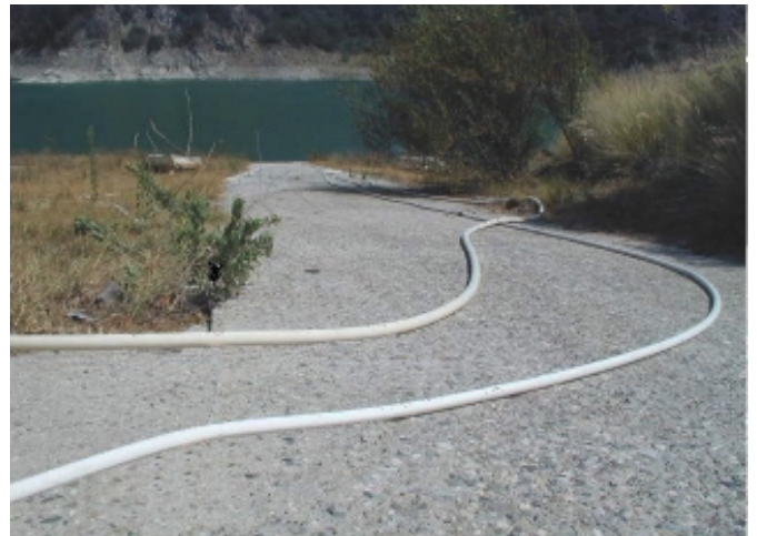
Figure 8—Ejector drafting operation at a sloped distance of 300 ft and vertical lift of 53 ft.
