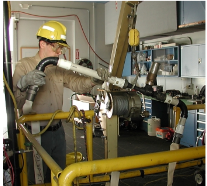
Figure 3—Positioning ejector test setup for dropping into well.
